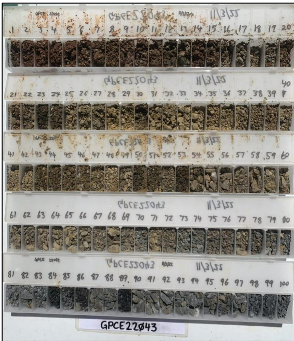
Figure 7: Photo of RC sample chips: Drillhole GPCE22043 1-100m
