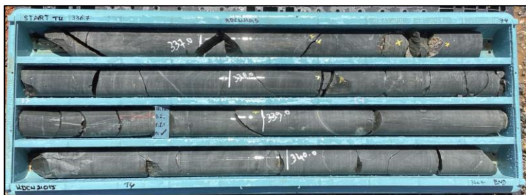
Figure 8b: Core for assay in trays: RDCW21015 336.70-340.40m (top = dry; bottom = wet).
