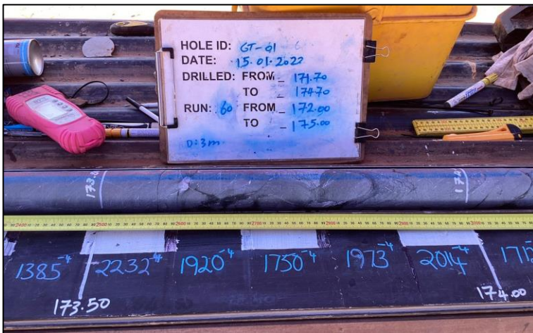
Figure 8a: Marked up core for lithology logging on the core table at the rig site (blue chalk numbers are magnetic susceptibility readings). The CormaGeo RT-1 Magnetic Susceptibility Meters used to take these measurements is at the top left (pink).
