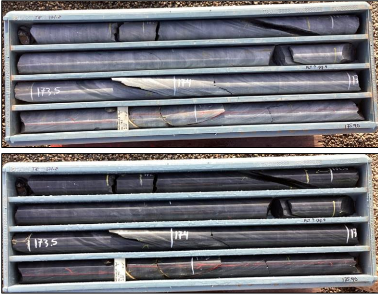
Figure 5: Photo of HQ3 geotechnical core: GPFO22047 171.80-175.90m (top = dry, bottom = wet). The core plug on the bottom flute denotes the information for the core run. Core plugs are also used to denote where lab samples are taken from.
