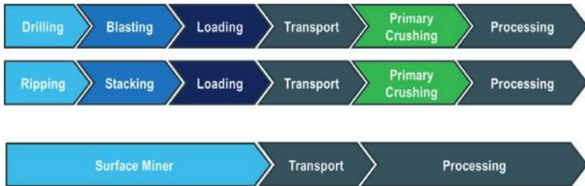
Figure 31. Comparison of process chains in open pits
