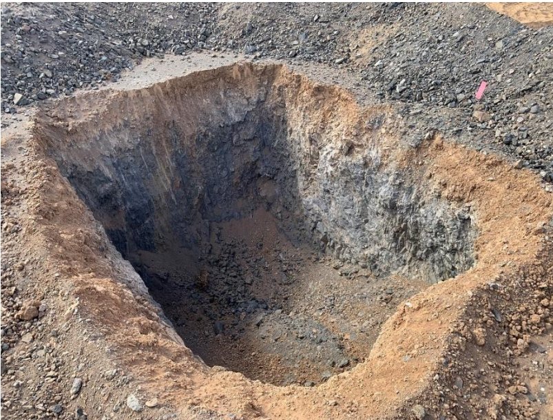
Figure 17: Very near-surface high magnetic susceptibility magnetitic siltstone sub crop was intersected while excavating the sump for drillhole RCFO23015.
