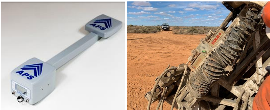
Figure 6: Rig and mast alignment via a Multi-wave Sensors GPS Azimuth Pointing System and a SOLA inclinometer.
